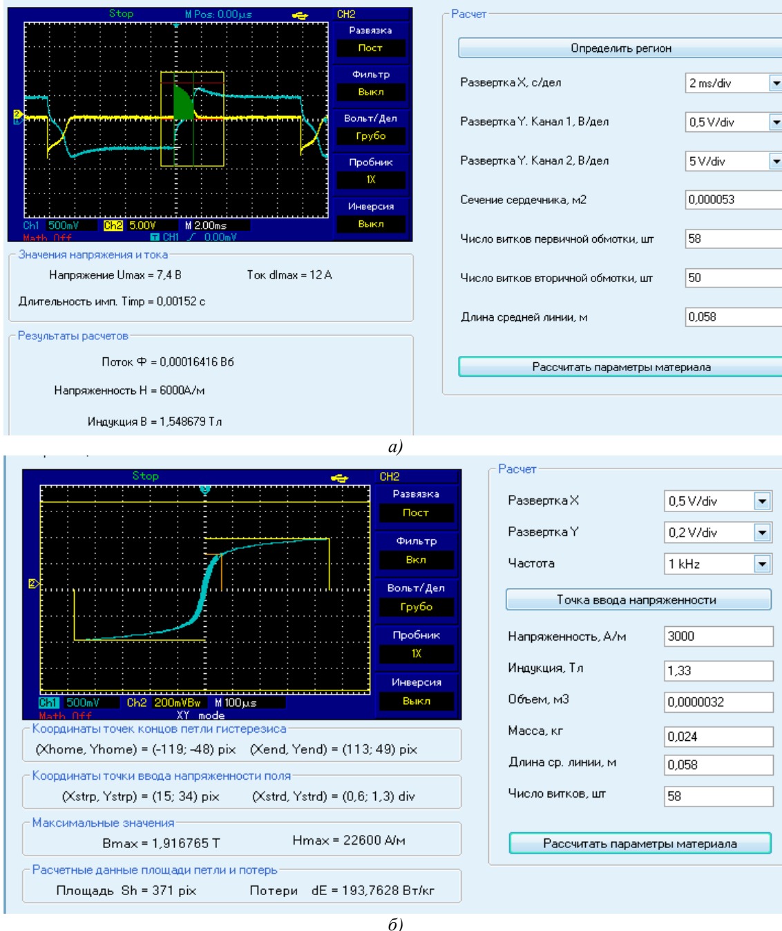
Figure 3. Results of data processing in the express flux meter (a) and express magnetometer (b) modes
